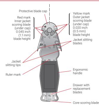
The nVent RAYCHEM Stripping-Tool-SR-Cable is designed for use with nVent RAYCHEM BTV-CR, BTV-CT, QTVR-CT, XTVR-CT, HTV-CT, HWAT, XL-Trace, IceStop and RaySol selfregulating heat-tracing cables. The tool is designed for faster, safer and more reliable cable terminations.
