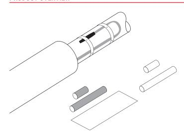
These end seal kits are designed for the termination of nVent RAYCHEM BTV, QTVR, XTVR, HTV and VPL self-regulating heating cables.
