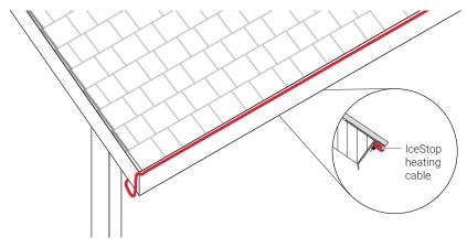
Fig. 11 Layout for heated drip edge
