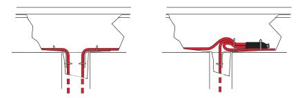
Fig. 16 Heating cable at top of downspout
