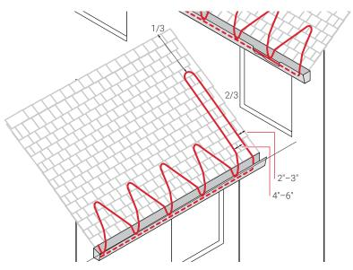
Fig. 13 Layout for a roof/wall intersection.
