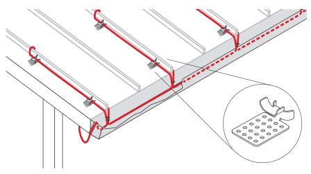
Fig. 19 GMK-RC clip on standing-seam roof
