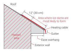
Fig. 6 Side view of roof with IceStop system
