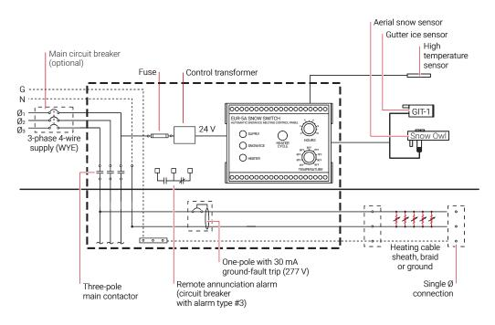
Fig. 27 Typical wiring diagram of group control with SMPG1
