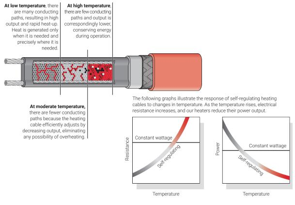
Fig. 3 Self-regulating heating cable technology
