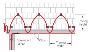
Fig. 5 Front view of roof with IceStop system
