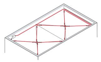
Fig. 22 Belt loop approach on a flat roof
