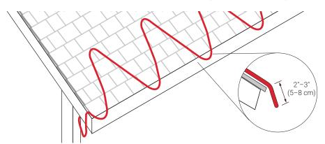
Fig. 10 Layout for heated drip loops
