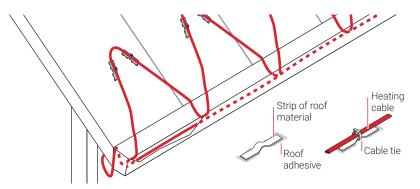
Fig. 21 Belt loop approach on a sloped roof
