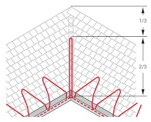
Fig. 12 Layout for a roof valley
