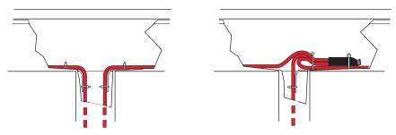
Fig. 24 GM-RAKE downspout hangers
