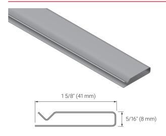
nVent RAYCHEM Cable Cover Bracket (CCB) is designed to mount on the roof or gutters and embeds one or two runs of self-regulating heating cable. It is used to enhance the heat transfer from the heating cable to the snow and create larger drain paths.
