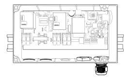
The nVent RAYCHEM HWAT-ECO-GF controller is designed for operation with the nVent RAYCHEM HWAT-R2 and HWAT-P1 self-regulating heating cables.
